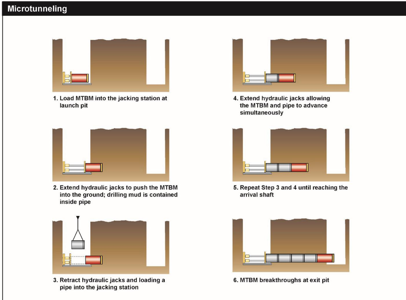
Figure 3. Appalachian National Scenic Trail Crossing – Microtunneling Process Drawing
