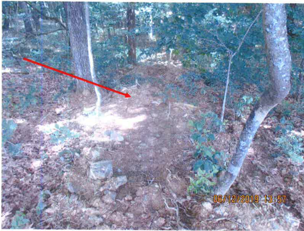
Below controls at station No. 9780+00 facing downslope at sediment deposits and scouring of leaf litter. Arrow depicts deposits.
