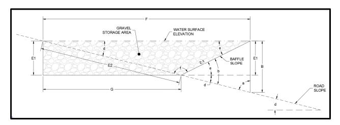
1. Determine the cross-section area (CSA) of storage behind each baffle, assuming a triangle based on bottom slope.
